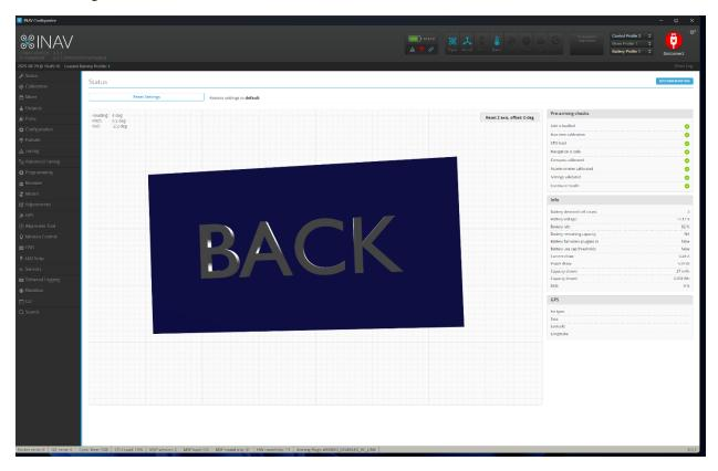
This is the "Settings" Page. The BACK picture represents the orientation of the flight controller. I changed the orientation in the "Adjustments" view to match the physical orientation in the boat.
