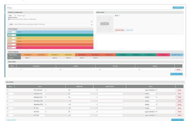
Servos 4 & 5 are used to control the "X" tail. They are used for both PITCH and YAW and are stabilized. The weighted values were derived empirically. Servo 3 is matched to "RC Channel 5" conditionally set by Logic condition 0 (defined in Programming). Servo 3 is also matched to "RC Pitch" in order to work with the X Tail Pitch movements. Servo 6 controls the Ballast Pump.
