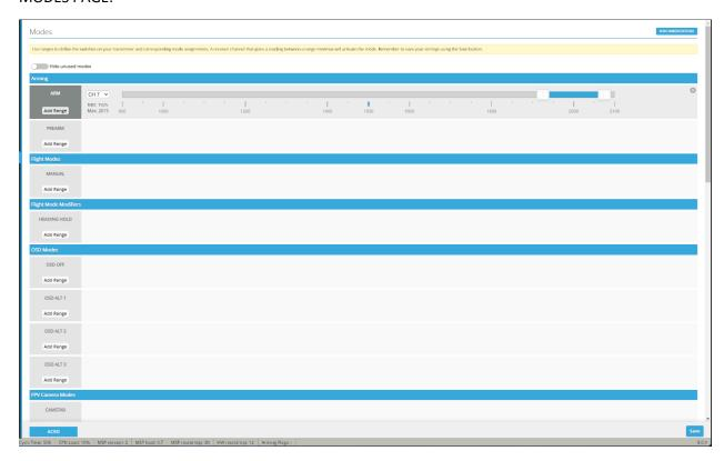
This page sets the Arming switch. This is a Quadcopter and airplane safety feature. I couldn't figure out a work around. The problems with arming were caused by a glitchy Tx switch. I now have a bit more confidence in this feature.
