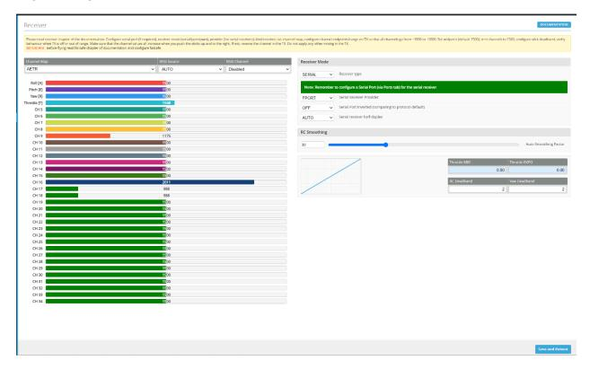
This page graphically displays the output values of the Tx. This is very useful for setup and debugging.
