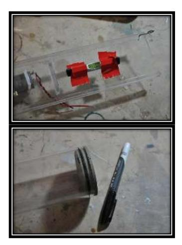
Once that is done it is time to put the tray into the WTC up to the mark that you made. It is also time to adjust the tray inside untill you get it level.
