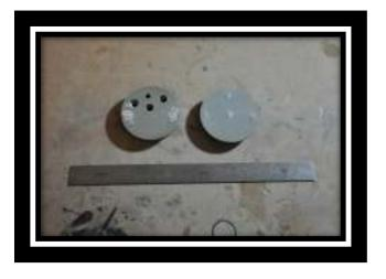
Once you have procured these items you will need to drill 3 holes in the end cap; one for the drive shaft and two for the push rod seals. The best way to determine what size hole you need is to get yourself a drill gauge and measure them. It is one of the best tools in my tool box.
