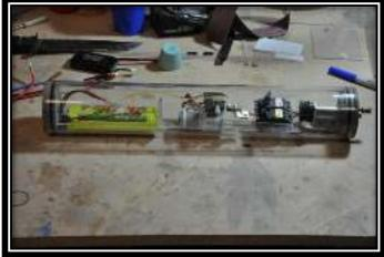
Now you need to drill a hole large enough for the servo cables to come through the tray to reach the RX. Pretty simple stuff; just make sure you don't drill the hole in Prime real estate. Also, take your time and drill small first and vary till your final size. Would be a shame to crack that tray at this point!
