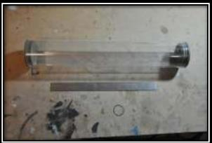
Now that the tray is cut to length you will need to trim it down to size so that it will fit inside with the rails attached. Cut two pieces of U channel to the length of your equipment tray. Place them on each side and try to insert the tray. Doesn't fit? File it down and try again. Rinse, lather and repeat until it goes in nicely. Make sure the fit is not so tight that it distorts the tube.
