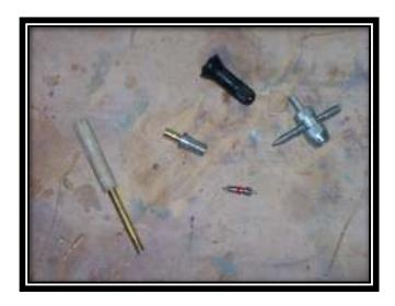
Next step you want to remove the valve so you don't damage it. That is because you will need to file the top (threaded side) of the valve down to make the inner pin more accessible to the servo swing arm for actuation. This is simple and I did it with a file. Just make sure you take it slow and don't take too much off. If you do you won't be able to thread the valve back in.
