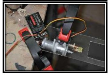
Next is to installed the servo (the micro servo)
