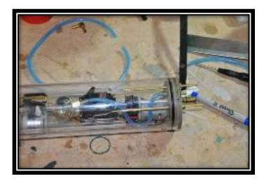
For the air tubes buy some aquarium hosing at Petsmart. It just seems to fit perfect. I also went to Ace Hardware and bought a 1/8" brass T fitting. This was so that the vent and pump could be connected in the same line. I also drilled a small hole to feed the hose through the equipment tray to the top. Make
