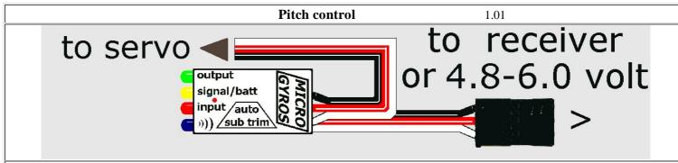
This pitch controller employs a high gain tilt sensor which will cause a servo to sweep its full travel with only a few degrees of tilt You may block this influence by connecting p1 and p2 together while setting servo to tiller arm linkage.
