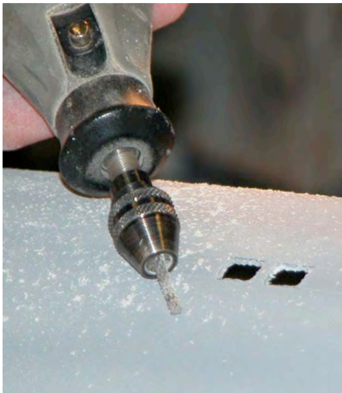
An eighth-inch diameter carbide burr cutter is used to both punch holes and do the rough shaping of
