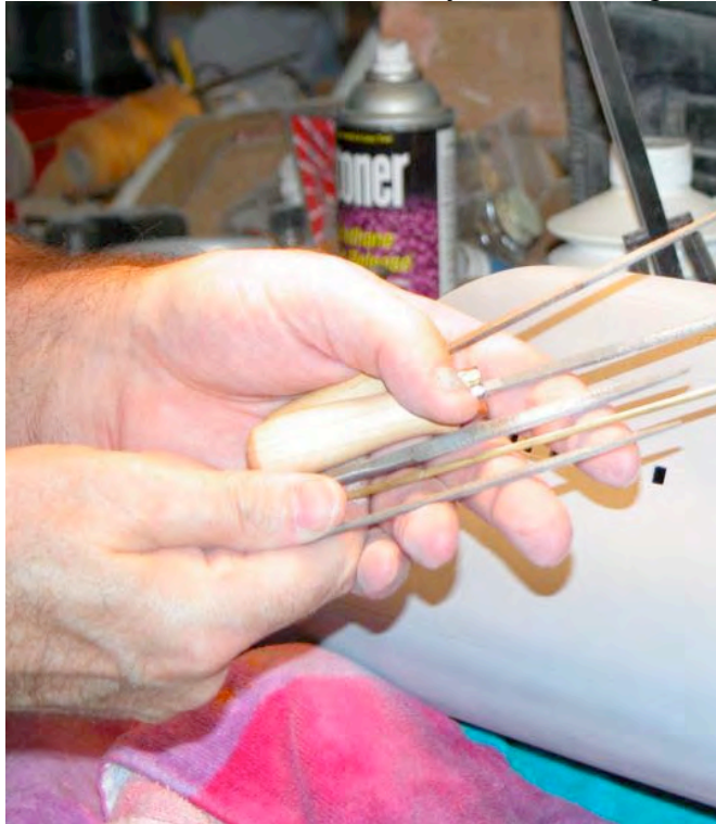
A selection of square hand-files used to rough out the many square holes that infest the ALFA hull.
