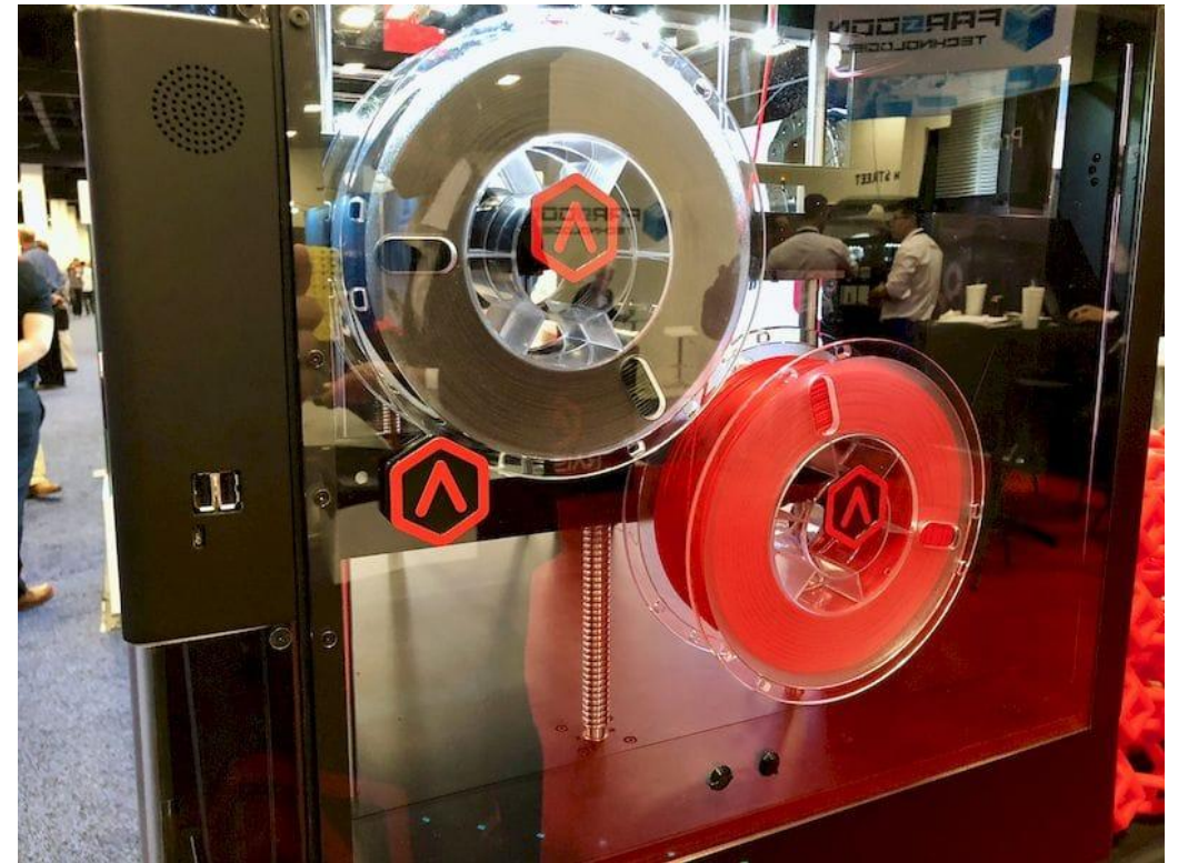
Dual-Spool Configuration on Raise3D Pro Series Printers
