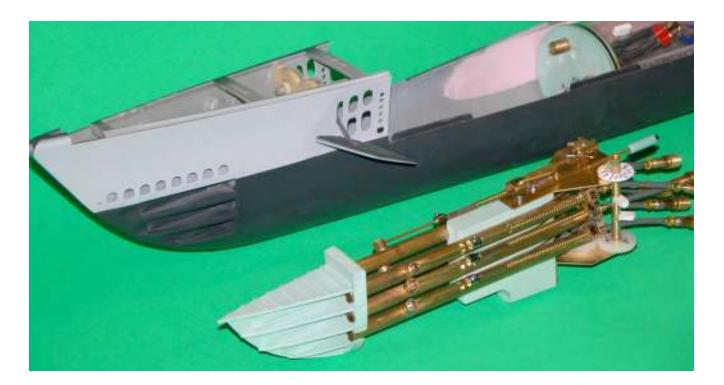
As you can see, things are a bit tight in the bow of the GATO with a complete set of launchers and the attached single-servo sequencing mechanism. Mounting of the four-tube nest at the stern of the GATO is done in a like manner.
