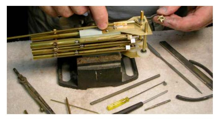
(You'll notice that the six launchers here employ spring-triggers instead of the shuttle button to actuate the launcher. The
