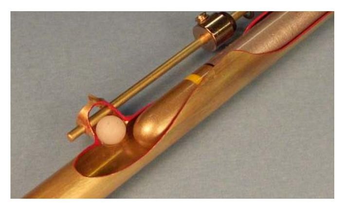
Note that the weapons nozzle makes a gas-tight union to the bore of the breech-block by the breech-block O-ring. The weapon can now be charged with a shot of propellant.
