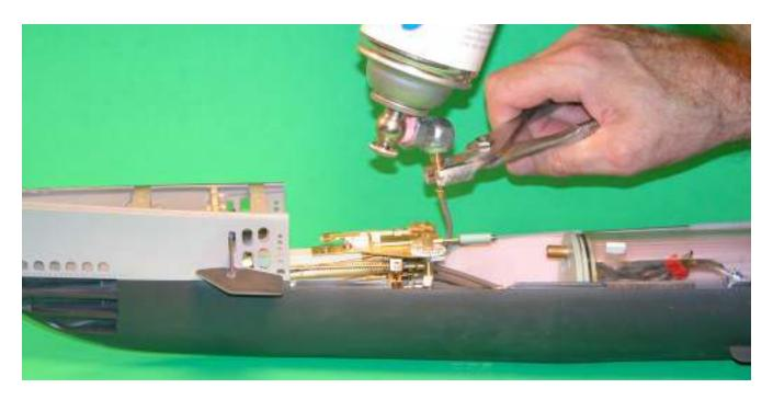
It's a good idea to hold the launcher charge fitting with the aid of pliers – this to prevent cold burns should too much liquid propellant spill by the charge fittings as liquid is transferred from can to weapon system.
