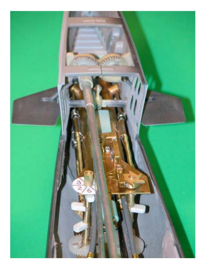
You must allow unobstructed after travel of the launcher flexible hose and attached charge fittings so that the launcher can transition from the battery to the launch condition. Any obstruction of that action could result in a jam, a miss-fire, when attempting to launch a weapon.
