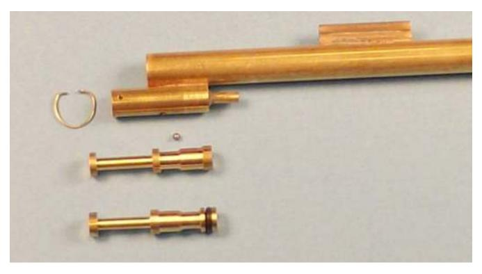
Only at the moment of launching, when the shuttle is moved (permitting the breech-block spring to shove the breech-block aft, and through the interlink rod, releasing the stop-bolt ball) is the weapon free to leave the tube.
