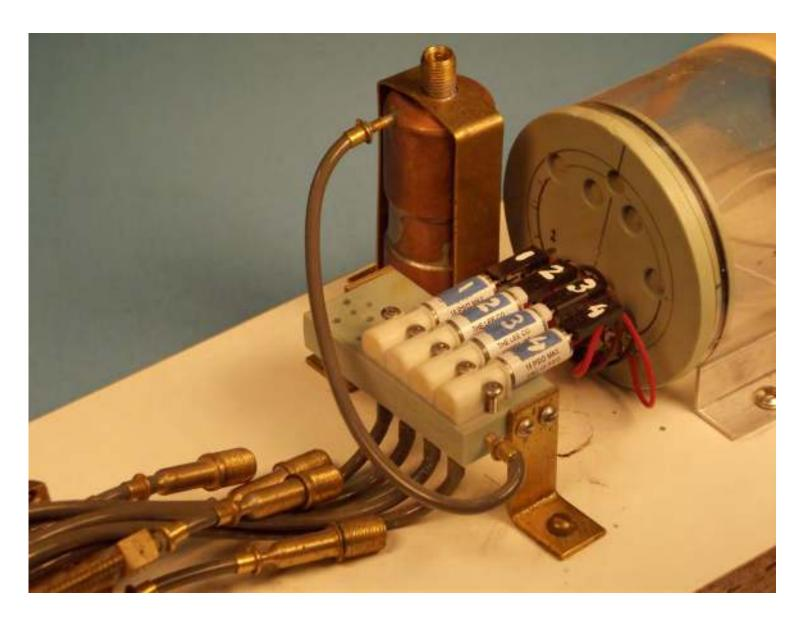
Threaded brass studs, that pass through the forward bulkhead of the SD, are the conductors between the wiring of the TCP (in the dry cylinder) and solenoids (in the wet portion of the hull).
