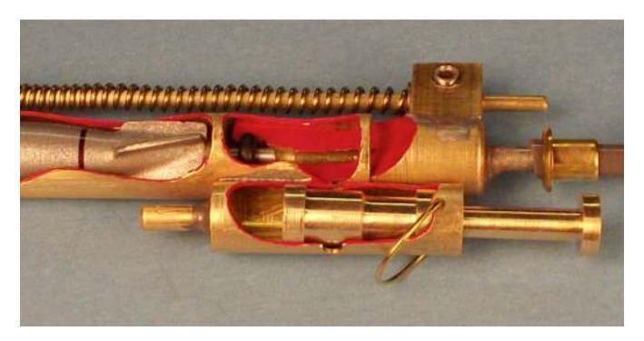
The photo below is a better look at the stainless steel locking-ball that holds the breech-block and stop-bolt ball elements to the battery condition. In turn, the locking ball is controlled by the shuttle beneath. When the shuttle moves in the desired direction it drops the locking-ball clear of the breech-block, permitting spring pressure to transition the launcher from battery to launch condition.
