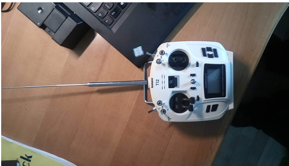
Figure 6. Another modern transmitter (Jumper T12) with the modified 40MHz JR module (top view)
