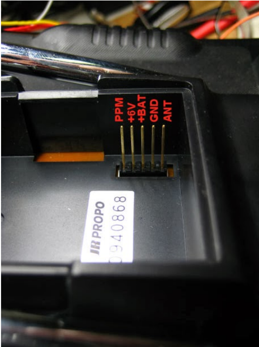
Figure 12. The assignment for the socket strip of the Graupner/JR 40MHz transmitter module in an old transmitter
