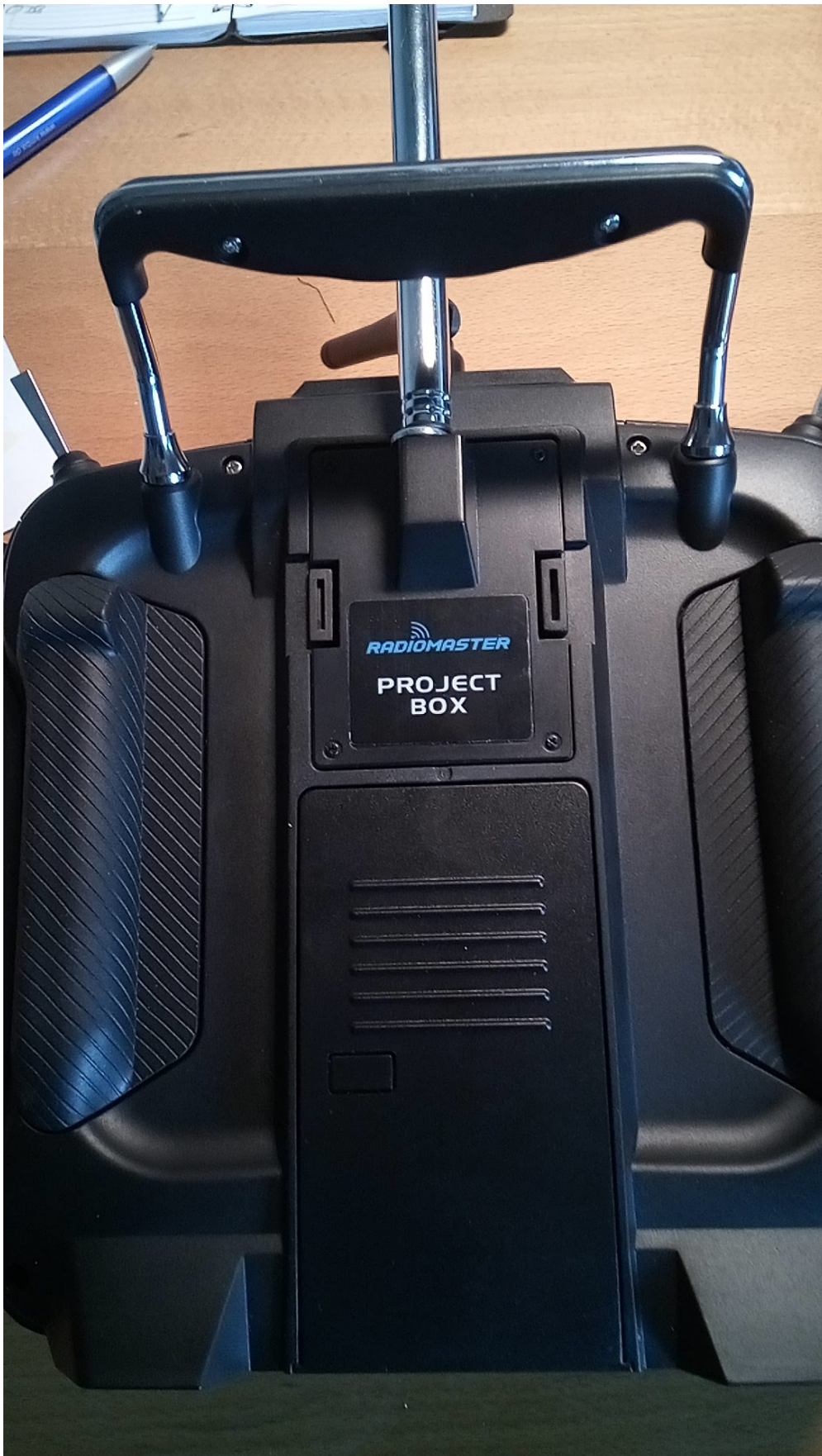
Figure 3. A modern transmitter (RadioMaster TX16s) with the converted 40MHz JR module (view: from below)
