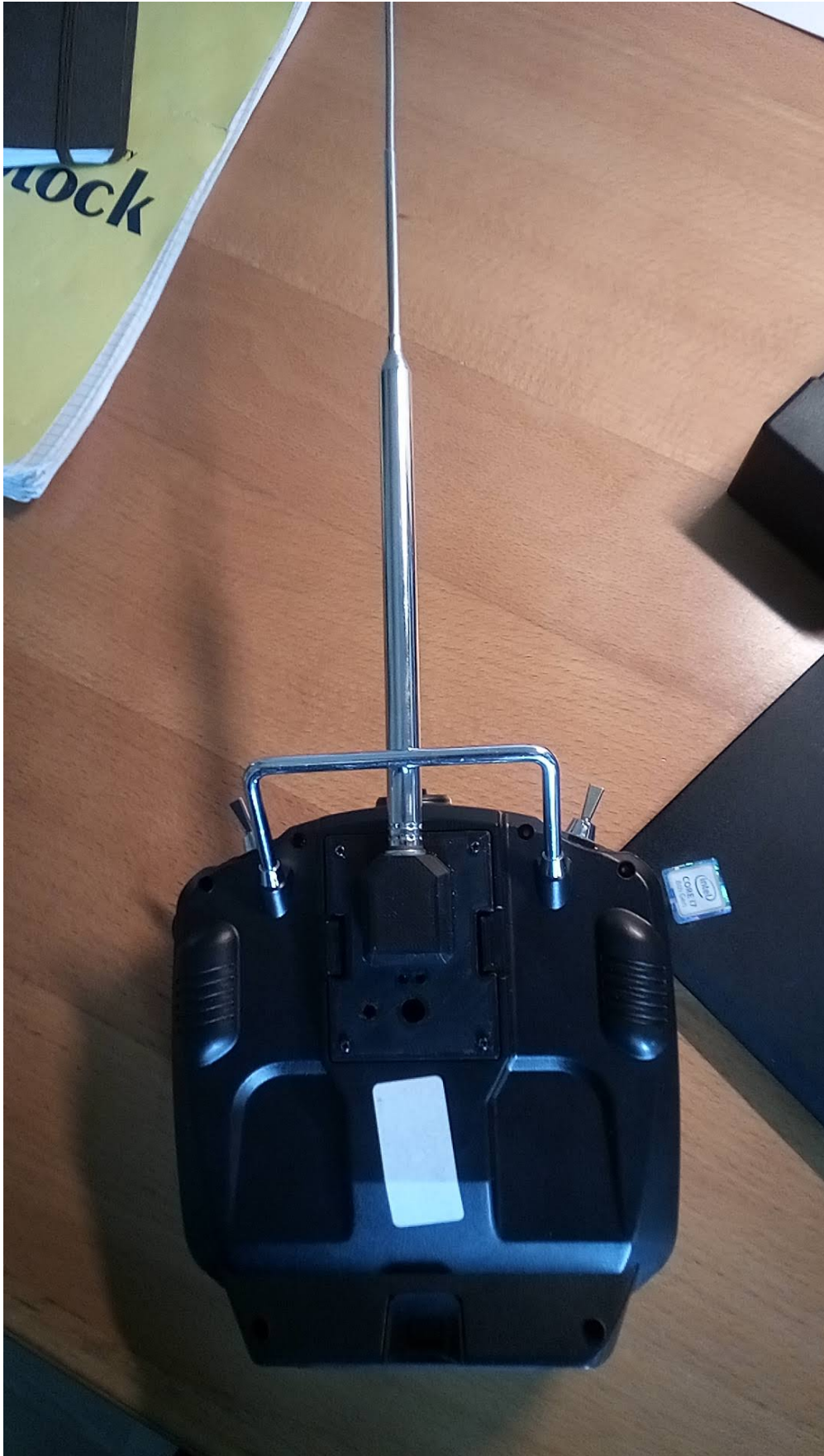
Figure 7. Another modern transmitter (Jumpe r s T12) with the converted 40MHz JR module (view: from below)
