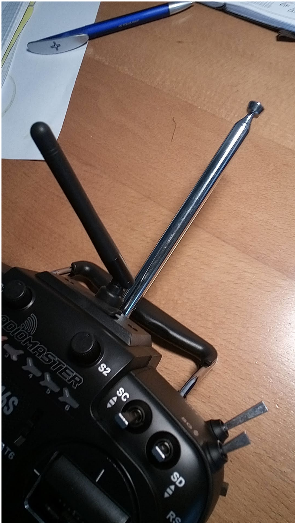
Figure 4. A modern transmitter (RadioMaster TX16s) with the converted 40MHz JR module /view: from above)
