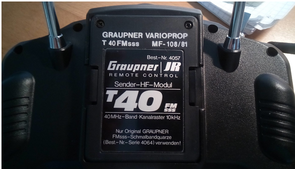
Figure 2. The mechanical dimensions allow plugging into a modern system (here: jumper T12). But: caution (see text).
