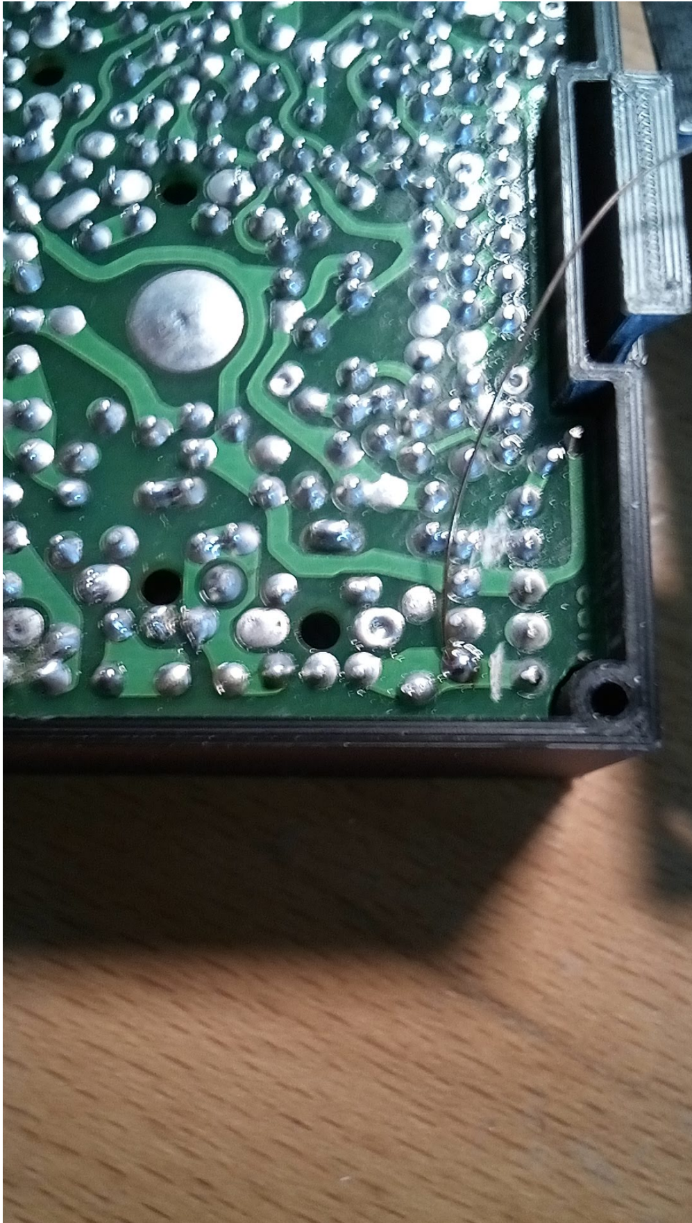
Figure 28. Extending the antenna signal with some enameled copper wire to the base of the antenna. Ensure good contact at the base of the antenna.
