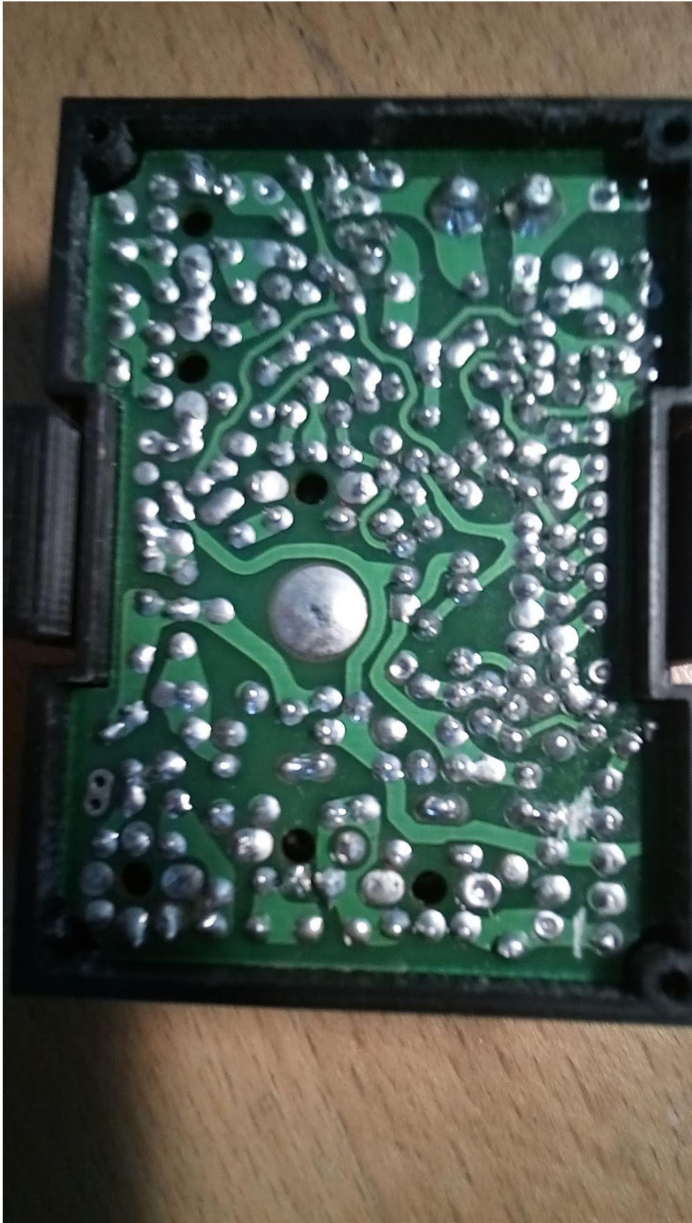
Figure 26. It may be necessary to adjust the circuit board with a Dremel (or similar) at the screw mounts.
